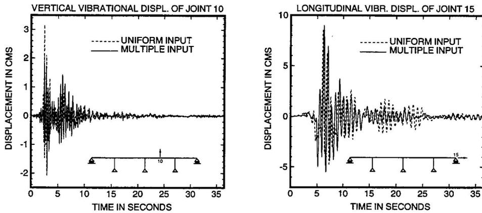
Figure 2. Time histories of the vibrational response displacements at joints 10 and 15 for the cases of uniform and multiple-support excitations.
