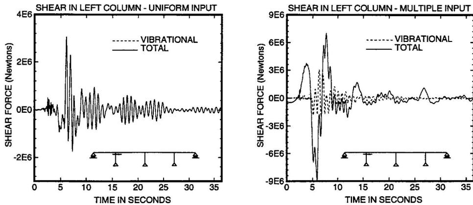
Figure 3. Time histories of the response shear force in the left column for the cases of uniform and multiple-support excitations.
